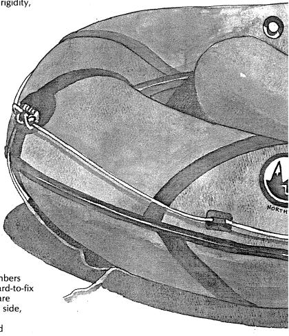
and buoyancy, and are formed as separate chambers before gluing into the boat to eliminate those hard-to-fix thwart seam leaks. The two main air chambers are formed at the front and back rather than side to side, because there's greater safety in this method of construction. Finally, all chambers have recessed military-style valves for quick inflation/deflation.
