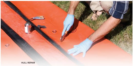
Your patch kit contains PVC boat material and Clifton Urethane Adhesive. You'll also need some type of cleaning solvent. PVC Cleaner (methyl ethyl ketone or MEK) is recommended; however, acetone or alcohol can be substituted. Adhesive and solvent have some toxic ingredients. Work in a well-ventilated area. Wear gloves and minimize breathing vapors.
