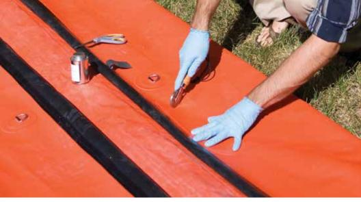
Note: Clifton Accelerator, item #38702.01.101, can be added to Clifton Hypalon Adhesive. It shortens the cure time and strengthens the bond. It is recommended for air holding patches and items such as D-rings that are subjected to heavy loading. We use this combination of adhesive and accelerator in the manufacture of your boat.
