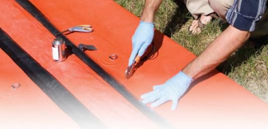
backside of the patch. Only scratch off the shiny finish of the raft material. Do not sand down to the point where the internal fabric threads are exposed. Use raft cleaner (toluene) to clean the repair area to remove any grease or oils and to prep the surfaces for best glue adhesion.
