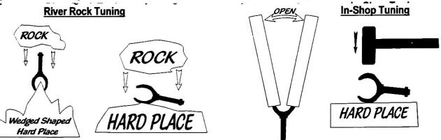
When tuning your fit, most experienced oar handlers like 1/8" to 1/4 clearance on the wrapped diameter. On the COBRA LOCK this should be observed mid-way up the opening (see split arrow).
