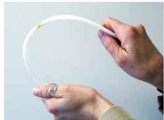
and splits in plastic canoes and kayaks. To test G/flex® for this type repair, we simulated splits in the bottom of a thermal formed plastic hull by edge gluing 1/8" thick high-density polyethylene (HDPE) sheets.
