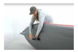
Remove the skeg from the bottom of the kayak, find a flat clean surface, and lay the Paragon down.
