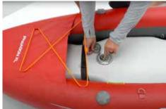
4. Deflate the three air chambers by pushing in the stem in the middle of the valve and turning it to the left (counterclockwise).
