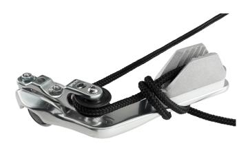
**Tech Tip:** If users need extra holding power for a larger anchor or heavier boat, looping the tail of the anchor line over the line between the cleat and pulley will greatly increase holding power and prevent accidental release of the anchor.
